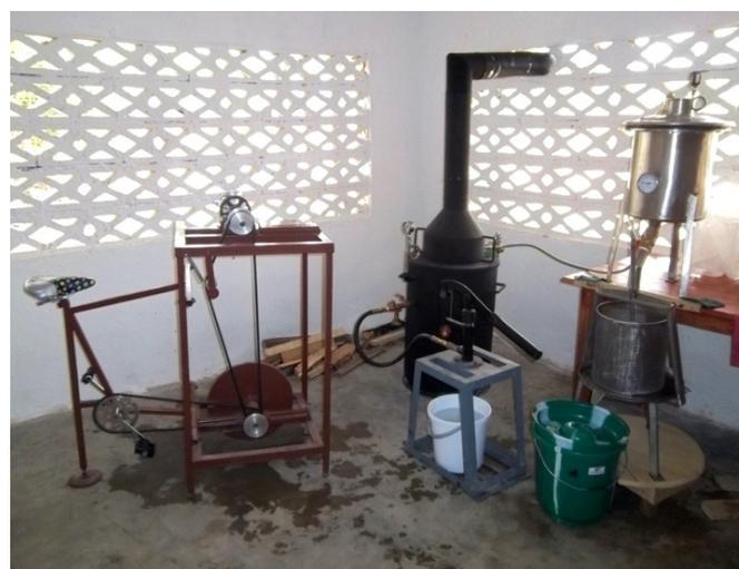
**Figure 5.** VitaGoat general components (left to right, top to bottom)<sup>8</sup>: Pedal-driven grinder, steam boiler, manual water pump, pressure cooker, and manual filter press.
