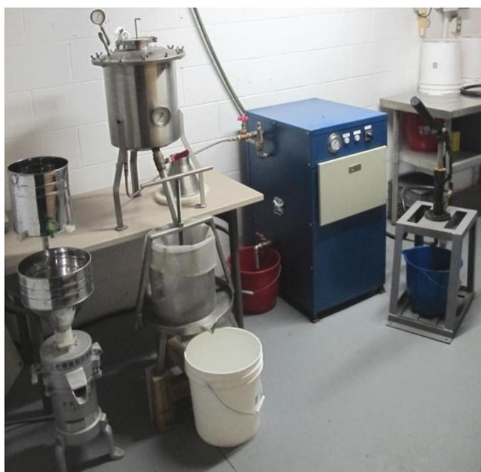
**Figure 4.** SoyCow “E” general components (left to right, top to bottom)<sup>22</sup>: Electric grinder, pressure cooker, manual filter press, electric boiler, and manual water pump.
