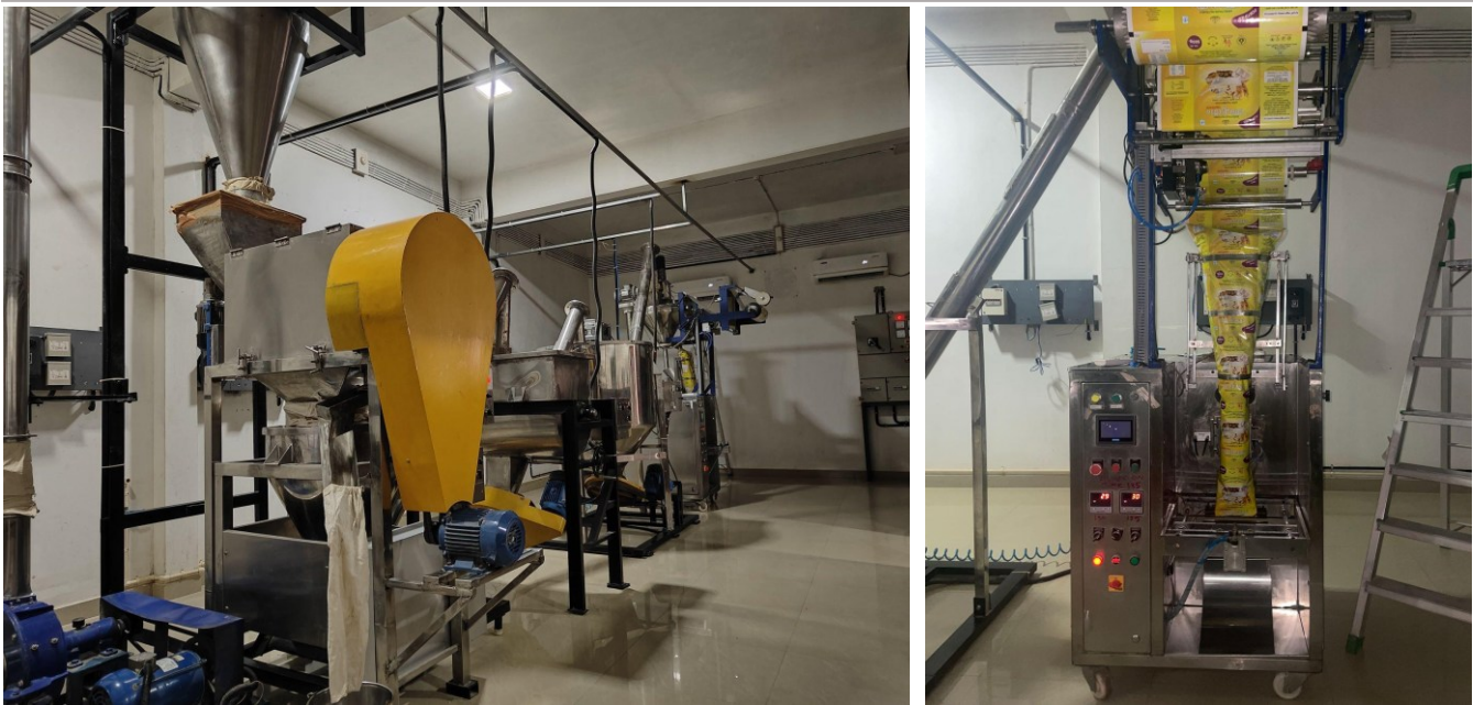
Figure 3. Manufacturing plant in Kottayam: grinding and mixing unit (left) and automated packaging machine (right). Photo courtesy of Kavya Dileep.
